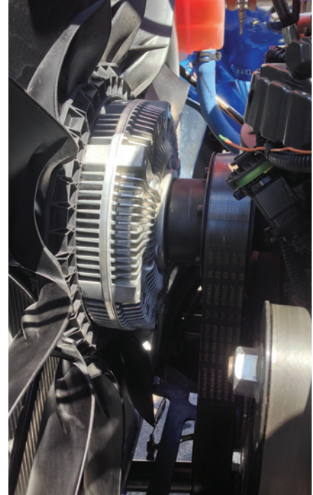
The RCV250 variable-speed fan drive installation
