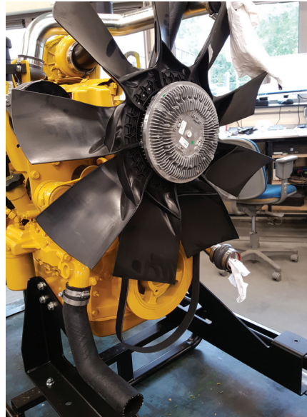
Front view of installed fan drive
