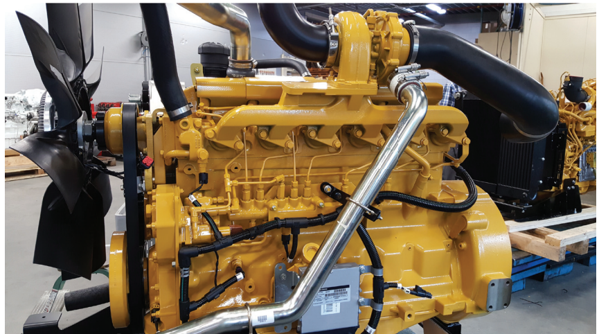
Horton VS227 Variable-Speed Fan Drive installed on John Deere 6.8L engine
